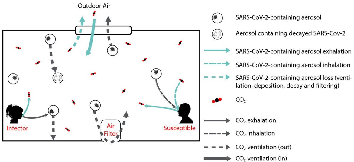
*Figure 1: Illustration of mechanisms for increasing and decreasing CO<sub>2</sub> levels and virus transmission in a ventilated indoor environment. The grey arrows denote movement of virus particles, and the blue arrows illustrate CO<sub>2</sub>. The mechanisms for decreasing virus particles are by natural decay and removal by ventilation or filtration. [1]*
