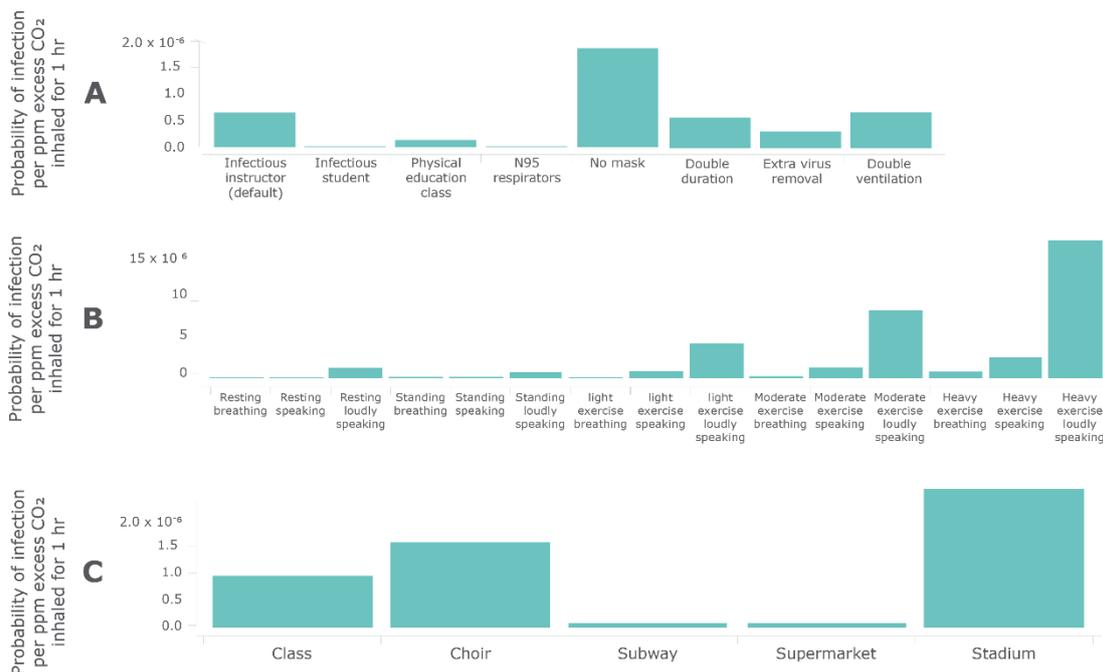
Figure 2: Probability of infection per excess ppm of CO<sub>2</sub> for a duration of 1 hour in different indoor environmental conditions. A: University class with 10 occupants, B: Varying levels of physical activity, C: Varying occupancy and room volumes. [1]
